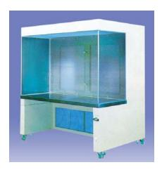
CLEAN BENCH is the clean equipment which enable you to create low cost clean environment for a particular area. It prevents the localized contamination at a particular spot. It creates unidirectional clean laminar flow at downstream of HEPA filter on the work bench. Two choices of clean bench: VERTICAL FLOW or HORIZONTAL FLOW.
